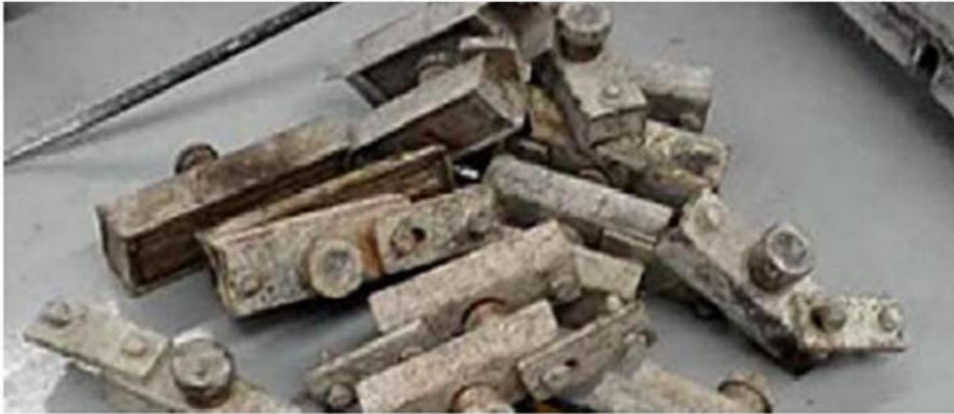
Rude discard shuttering magnet lead to deformation
