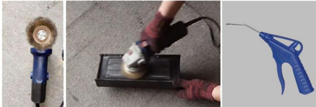
Shuttering magnet bottom debris is not cleaned
